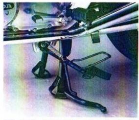
A sturdy main stand and a handy side stand are fitted, the side stand with safety guard, rubber tab to retract it if forgotten.
